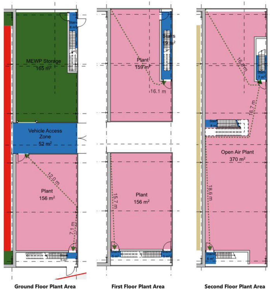
Figure 2—4 Travel Distances in the Plant Areas
