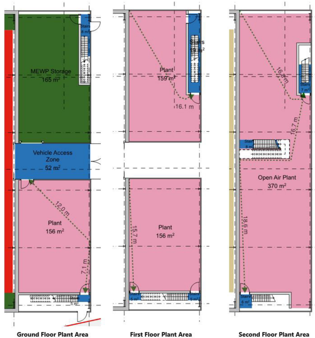
Figure 2—4 Travel Distances in the Plant Areas
