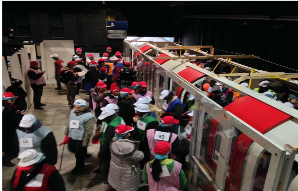
Figure 2—1 Example Experiment Set Up in the Current Facility. Mock-up Train Unit and Platform Edge Doors Made from Plywood (with Polycarbonate Glazing in the Platform Edge Doors, but Open Windows in the Train).
