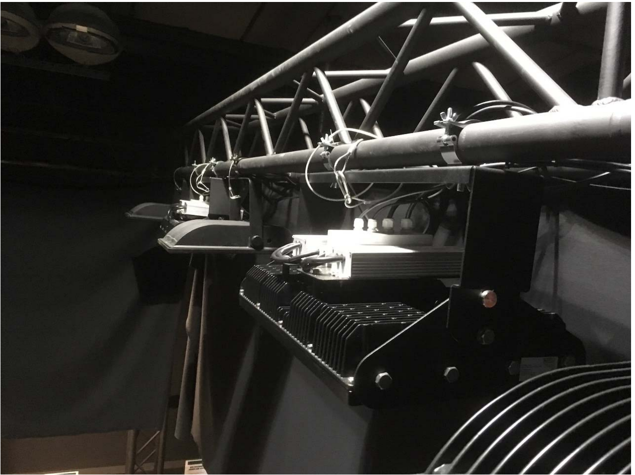
Figure 3 Upper side of lighting units: foreground: high powered white unit; Rear: colour unit
