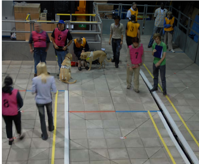
Figure 7 Experiments with visually impaired people to explore different ramp gradients for the Victoria Line Upgrade
