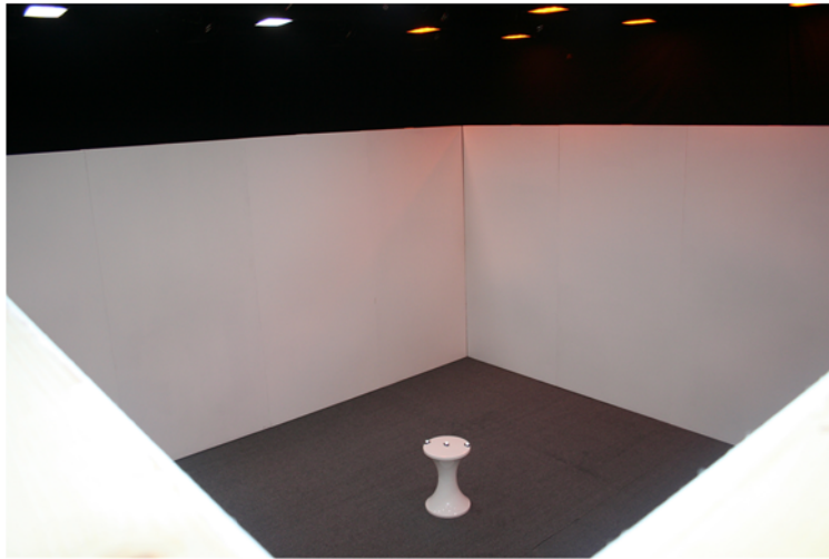
Figure 8 A neurology experiment where spatial memory is being tested. In this case, a featureless room is set up (framed plywood panels) and the size and shape of the room is changed during the experiment.
