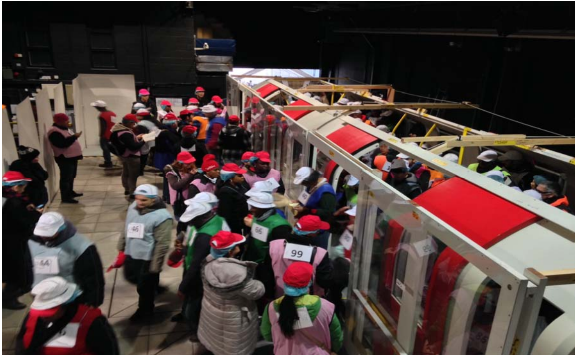
Figure 5 Mock-up train unit and platform edge doors made from plywood (with polycarbonate glazing in the platform edge doors, but open windows in the train). We would not be expecting to have such a mock-up in PEARL as we will have actual (steel/aluminium) train carriages stored outside for most purposes, but it is possible that we would need to create and store a new design mock-up (as in this case where the research was about a new innovative design). This also shows some plywood panelling used to screen off the 'platform' rear edges. These are made from 3 ply (as can be seen in the photo, the train and doors are made from much thicker 15-20mm ply). We are expecting the large scenery sets (e.g. 100m long street) to be much more substantial than this, with steel reinforcement, and representing the 3D environment of a street frontage (i.e. incorporating window sills, doorways etc.). We operate these experiments with a number of assistants (ratio 1:10) for health and safety reasons.
