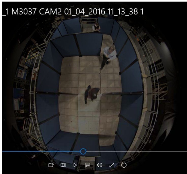
Figure 9 A simple maze set up for an Ophthalmology experiment under low lighting levels. The maze is constructed from standard temporary screens, arranged as required.
